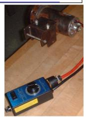
Murray's Auto Parts. The motor is a 2-1/4HP 120Volt DC, and he got a Harbour Freight variable speed AC controller and added a rectifier bridge to control the DC motor with 120Volts AC, controllable from about 25 to 3000 RPM. Works slick for very little cost, and is very powerful. He thinks he will install it on a drill press.
