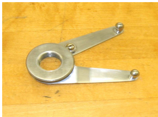
A very nice dividing head quadrant under way.
