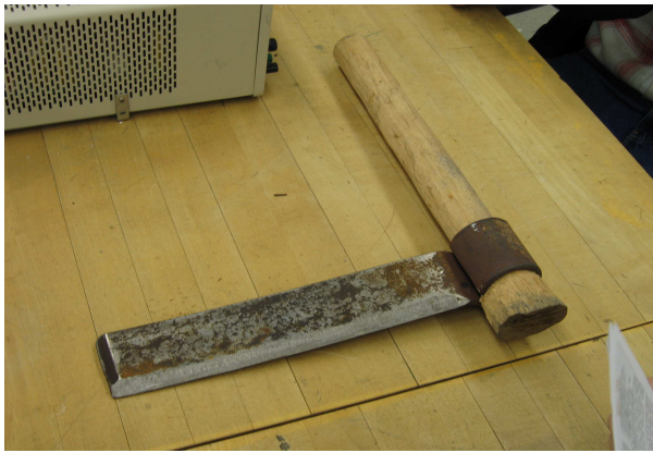
Log-splitter from a car-spring, for the wood-pile.....
