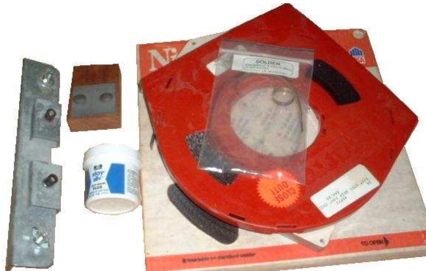
Larry Williams brought in these fixtures, silver solder and band saw blade material. He explained how he tried every method available over a long period of time to make his own blades. His final solution: the fixtures above, a scarf joint in the blade and silver solder. He has never had a blade break at the joint with this method. He also showed how to coil blades by standing on the blade and push down while turning the hand.
