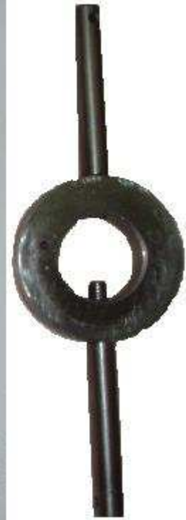
Emil brought in two items. The drawing is of a vortex tube (one end blows hot air and the other end blows cold, very cold air). The item on the left is a device Emil uses to turn taps by hand in his drill press. The lower handle goes into hole for the chuck key and holds it in place.
