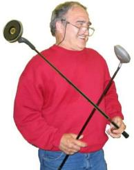
**Bert Campbell** with another dandy. He bolted a welding "ground-clamp" magnet through an old golf club head. Put a plastic bag on the magnet, pick up chips, peel the bag off inside out, and voila!! Clean magnet! Bag full of chips!!
