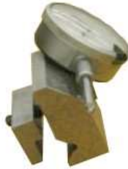
Emil Caffarelli’s neat and simple DTI holder to clamp on the lathe bed. Photo doesn’t show the superb “frosted” finish on the base. Another beauty for Emil!
