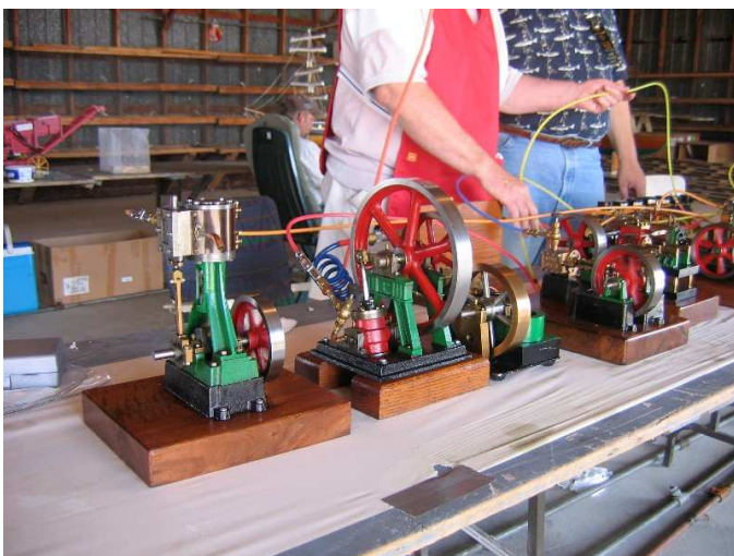
A whole table of the group's fine workmanship, all turning silently,.... on air pressure of only 7 PSI. Wow!!! And that also included ....
