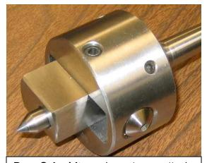
Ron Schmidt made a taper attachment for the tailstock of his lathe – from an old boring head. He turned down the R8 shank to a #2 Morse and put a lathe center in place of the boring cutter. Nice.
