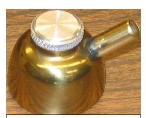
Emil Cafarelli made a cute alcohol burner from a hollow doorknob and a brass tube in about an hour. He is obsessed with how the doorknob was manufactured. Can someone say definitively so we can put this matter to rest?
