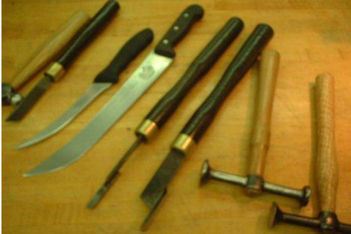
Thess are from James' toolbox. All were sharpened or reconditioned with his belt device. You can see James likes making his own handles too
