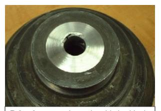
Brian Lawson showed us his bad luck. He broke his 5-step pulley and looked for a replacement – for about 10 hours – but found none. So he worked for a ½ hour to make it into a 4-step pulley, but just when he thought he was home free, he discovered a void in the casting right where the setscrew needed to go. I think he said "oh, shucks, isn't this amusing…", or something like that.
