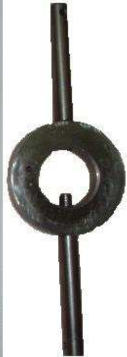
Emil brought in two items. The drawing is of a vortex tube (one end blows hot air and the other end blows cold, very cold air). The item on the left is a device Emil uses to turn taps by hand in his drill press. The lower handle goes into hole for the chuck key and holds it in place.
