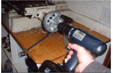
**John Osborne** (me) brought in a device to turn the hand wheels on my mill. But without the mill and the drill it chucks into, it was hard to visualise what it did. I use this like a power feed for X and Y feeds and for rapiding between cuts.
