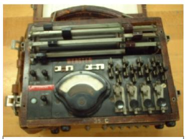
**Bob Fuhrman** "rescued" the object above from the trash .He said it was too good for the junk pile. I agree. It's a fine old relay adjustment kit. Its used to check and adjust precision relays to current in milliamperes.
