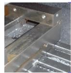
John Osborne I got frustrated with the bolts holding down the vise. They are hard to clean around and got in the way when hanging work pieces off the side of the vise. Drilling holes for cap screws running into T-nuts took care of that.
