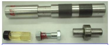
More LocTite stuff. This shows metal repair and retaining compounds, as well as threadlocking and how some pipe sealers can get into the oil.
