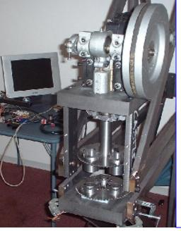
John Osborne here again. I am rebuilding my punch with a flywheel to get about 10 times the punching speed of the servo system. You can see a turret for the punch holders and one below it for the dies. Roller chains will sync the two turrets. I hope vou fellows don't mind me putting this in the newsletter, but its too big to bring in.
