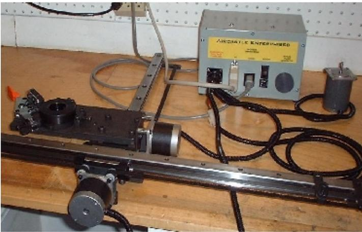
This is another CNC punch I built after the flood. The customer already had the hand punch I normally convert, so I built the rest of the system. The grey box has the interface, power supplies and stepper motor drivers.
