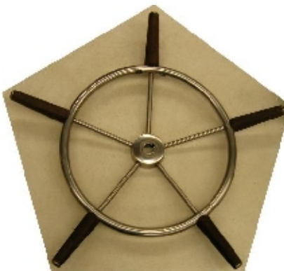
Joe Pietsch demonstrated a $7 ship's wheel, a great piece, incidentally, which he uses as the operating wheel to raise and lower his drill press quill. It performs that function perfectly and elegantly.
