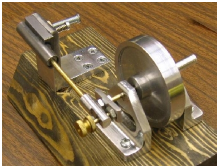
James Hagle demonstrated a small air engine he developed from a similar steam engine purchased at a garage sale. He made at the M.C. College classes he took there.
