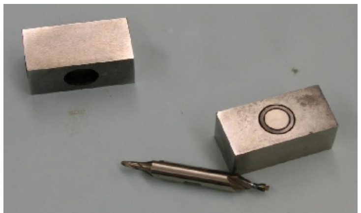
Jim Howard had a few items from an auction that he asked the guys to help him identify. The 3/16 end-mill has a flute that is stepped and the two ground pieces have re-locatable magnets.
