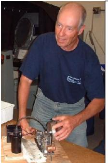
Karl Gross showed his hit and miss engine in operation. It is called because that the ignition is cut off when the engine exceeds a set speed. (It's a heat engine, I know that now. Emil).
