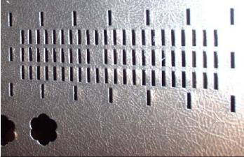
**Your president** has finally finished the CNC punch! This is a test piece, which was punched in about 28 seconds at a rate of about 3 punches per second. Its fun to watch.
