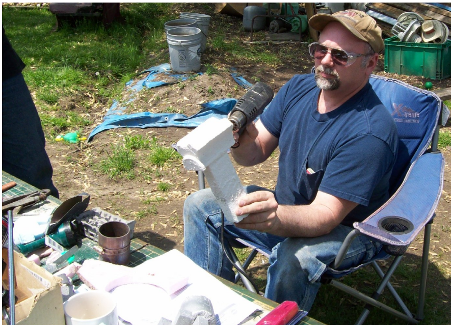
Steve Huck glued together three layers of styrofoam, cut out freehand an engine block using a hotwire cutter, coated the pattern and dried it with a heat gun. Rick used his aluminum casting magic and whala !
