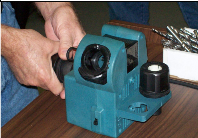
Rick's Garden Structure, note the curved ends which was done on a CNC. Phil Shannon demonstrating the Drill Doctor. The Drill Doctor and the collet used to hold the drill bit. Another attachment for grinding drill bits and some large drill inserts brought in by Brian.
