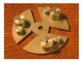
Of course, Phil's version was MUCH nicer! The spider is placed on the face of the chuck and a ssists with flat clamping of thin m aterials for facing. The safety advantage of the spider over using parallels is that the spide r is captured by the chuck jaws. Thanks for the tip Phil!
