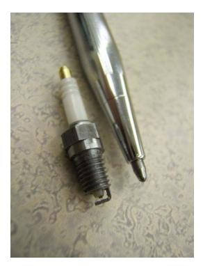
Joe Pietsch shared a v ery unique glass cutting tool from his collection. It has a finely adjustable depth control and is used to make internal cuts on glass tubing for use in boiler construction and maintenance.
