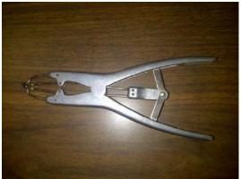
This tool can be found at places like Tractor Supply Com pany or Farm & Fleet stores. The business end uses four expanding fingers which stretch the Oring when the handle is squeezed:
