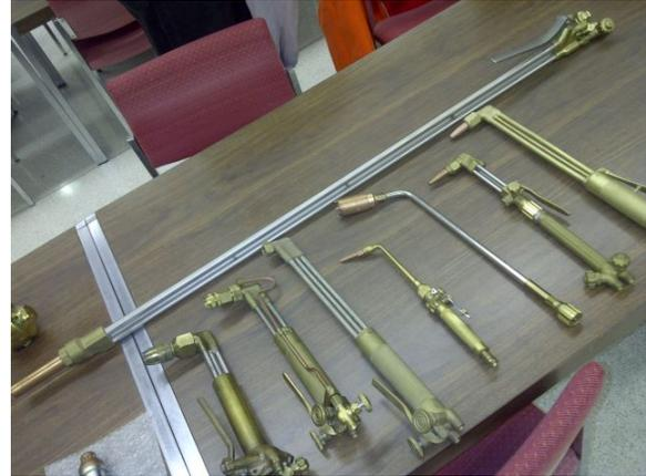
David made a monumental effort to bring along an impressive collection of equipment. The longest torch, at the top of this photo, is a little over 4-feet long and is capable of cutting through 5-feet of steel.
