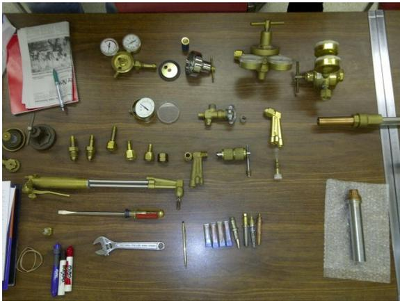
Dave gave some pointers on identifying the different types of regulators, fittings and brands of equipment which are capable of being refurbished.
