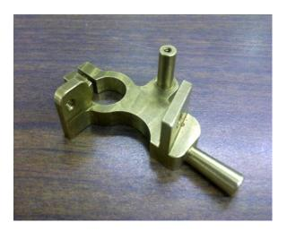
Here is another view, oriented upright. The top stud is a lever used to vary the ignition timing while running:
