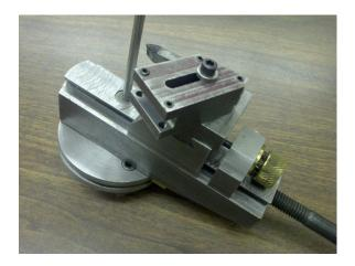
It mounts to the cross slide and can turn an inside or outside radius:
