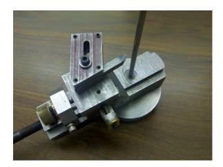
The device is thumb screw adjustable for cut depth control. It operated very smoothly, no doubt to Louie's fine craftsmanship. Kevin Thomas brought along the crankshaft of his Panther Pup engine. It was turned from 5/8 bar stock and was nicely detailed:
