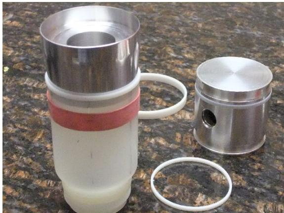
George explained in a post-meeting email that “the thin section allows the seal to pass over the wear ring groove, the plastic bottle piece with slots is the "pusher".”
