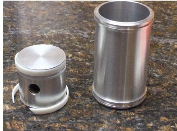
During the meeting George discussed the difficulties of securely holding a finished-machined piston so that internal snap ring grooves could be accurately cut to retain the piston pin. He developed this mandrel, which he reported worked well –
