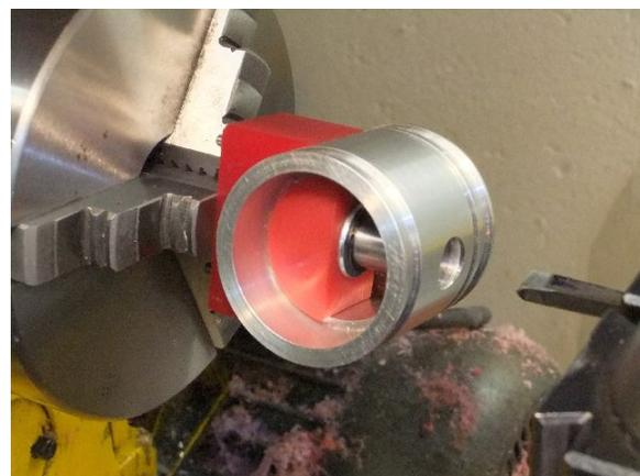
Kevin Thomas suggested using an expanding arbor within the piston pin hole. This method would improve concentricity between the pin axis and snap ring groove.
