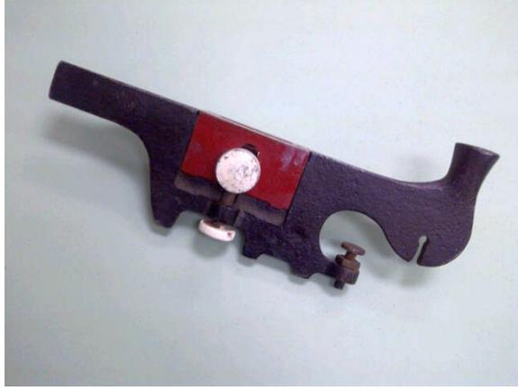
It has multiple functions as a hammer, tooth bender for adjusting the “kerf” (width of the cut), gage, sharpening guide and probably other uses. It was patented in 1885 and probably commonplace in Michigan’s logging heyday –
