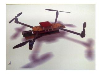
His new machine will use a birch ply body and carbon fiber booms for weight reduction and strength –
