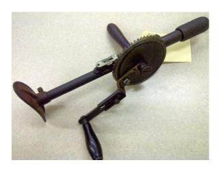
Some of the braces had two speed settings. Here is a close up of the same Miller Falls No.12 from above showing the bubble level and back side of the drive plate with two bevel gear of different circumference –
