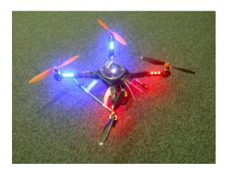
This big machine was remarkably stable during flight. Ted controls the throttle and direction, while the rotors and gyro are processor controlled to give the machine good gust resistance at altitude –
