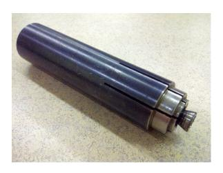
Kevin suggested then, and now, that an arbor of this type can be turned to close tolerance with the bore diameter within which the groove needs to be cut. The arbor's tapered screw head then expands the device evenly to ensure concentricity –
