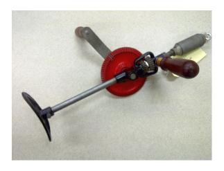
The following brace was also made by Miller Falls. It is a No.980, made from 1925-1930. The frame is intricately cast (like the No.119-A above) as is the drive wheel –
