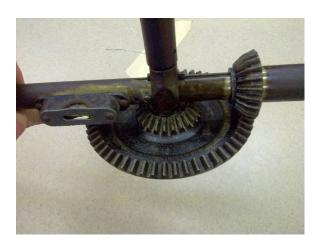
This next brace is a Miller Falls No.77, made from 1938-1948. The supporting handle-side pinion bevel gear is visible from this position –
