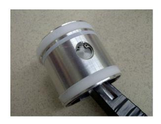
Slightly less obvious is George's careful attention to friction reduction found *inside* the piston skirt. The gudgeon pin rides on a roller bearing (also retained by snap rings) instead of the usual bronze bushing –
