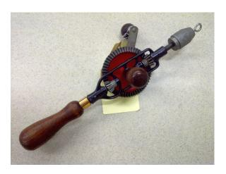
The following brace is a Miller Falls No.119-A, made from 1938-1962. It was a contemporary of the No.77 above, but appears to have several different features which set it apart in the manufacturer's line up –
