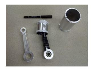
The rod with the piston is taped to protect the beam and cylinder during trial fits. At previous meetings (see the January 2013 MDMC newsletter) George discussed a jig that he developed to cut the gudgeon pin retaining ring grooves. The technique was successful, the nicely cut groove being seen in this assembly –
