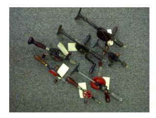
This first model is a Goodell Pratt No.655 hand brace, patented in 1895. The casting around the gear work is intricate, and it has a pinion bevel gear on the handle side to help stabilize the drive gear –
