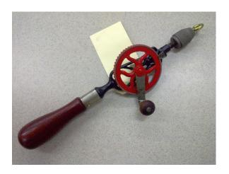
This next model is a Miller Falls No.12 (made from 1925-1931) with a breast plate and another intricately cast frame. The drive handle arm can
