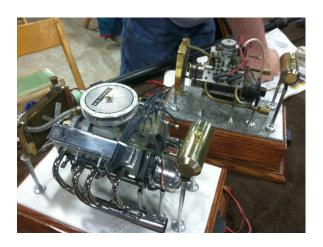
For instance, between NAMES 2012 and 2013, Steve managed to put together this V-twin I.C. engine based on an air compressor casting for the cylinders and block, but with *everything* else of his own design:
