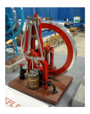
Jerry also modeled an engine made by the Kimble Engine Co. of Kalamazoo. It is a unique design, having "no piston, crosshead or ways":
