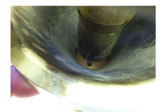
... to keep the metering flow sonic and, therefore, more consistent. The goal was better atomization, leaner mixtures, and lower emissions. The design was issued patent #4000225, but was not adopted commercially because of difficulties with operating under a wide range of environmental conditions. For instance. Jav mentioned that changes in humidity disrupted the sonic shock wave, which altered the intended fuel/air metering circuit. Thanks Jay for sharing this very interesting device!
