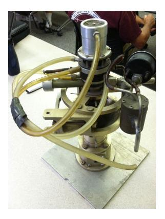
The carb sought to take advantage of the independence of sonic flow from variable manifold pressures in order to provide more even fuel/air metering. A cone shaped venturi "restrictor" could be moved ...
