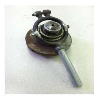
Jay Druillard brought in an experimental "sonic flow variable venturi area carburetor":
