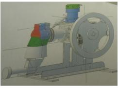
George took us through the details, complete with cad drawing and tooling, of how he designed and built the stainless steel ducting that will be used on the Stirling engine he's currently building. In the photo to the left, the ducting shown on the left concentrates the heat, from the source, onto the heater cap. Below on the right you can see the forming dies that he made up and used to form the fastening holes, increasing the surface area of
