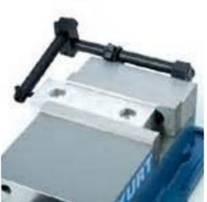
machining practice. A quick video appearance by Tom Lipton shed some clarification on just how far, or not so far, out a vice jaw can get when clamping up a small part on one end of the vice. The angle can be relatively small, but there, when this easy preventative measure is skipped. Bottom line - you need to know your machine, your vices, the part and the machining operation being performed in order to make an informed call on if, how and when to use a packing set up.
