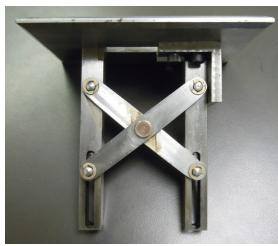
tackle. The set up fits in the regular jaws of your vise and when you apply clamping pressure with the vise jaw, it is translated to the small jaws shown in the above picture gripping the smallest of items, thin sheets of metal etc.... Thanks Brian!
