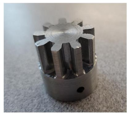
Club President Steve Huck presented on his process for making gears with his CNC mill using an end mill. He brought along the small gear produced using this process, shown at left, for show and tell.
